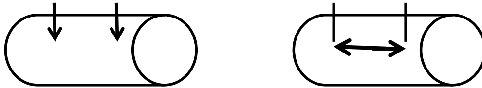
Figure 2 Schematic of Monitoring (a) Point-to-Point and (b) Along the Length
