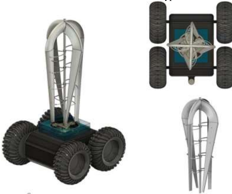
Figure 4: Proposed mobile wind energy unit.
