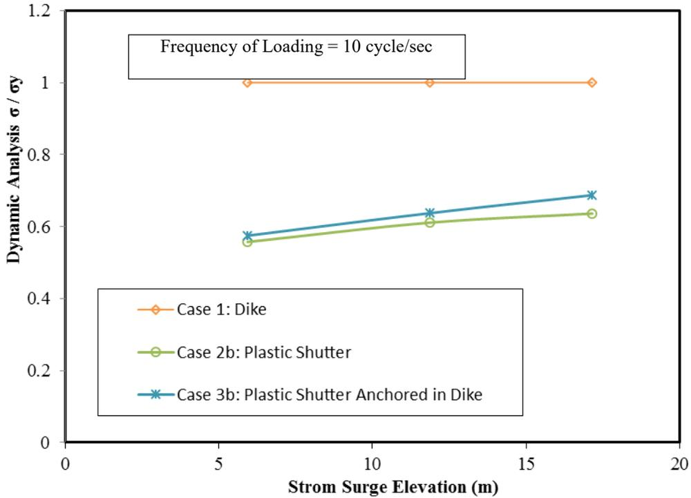
Figure 24: Normalized von misses from dynamic analysis versus storm surge elevation
