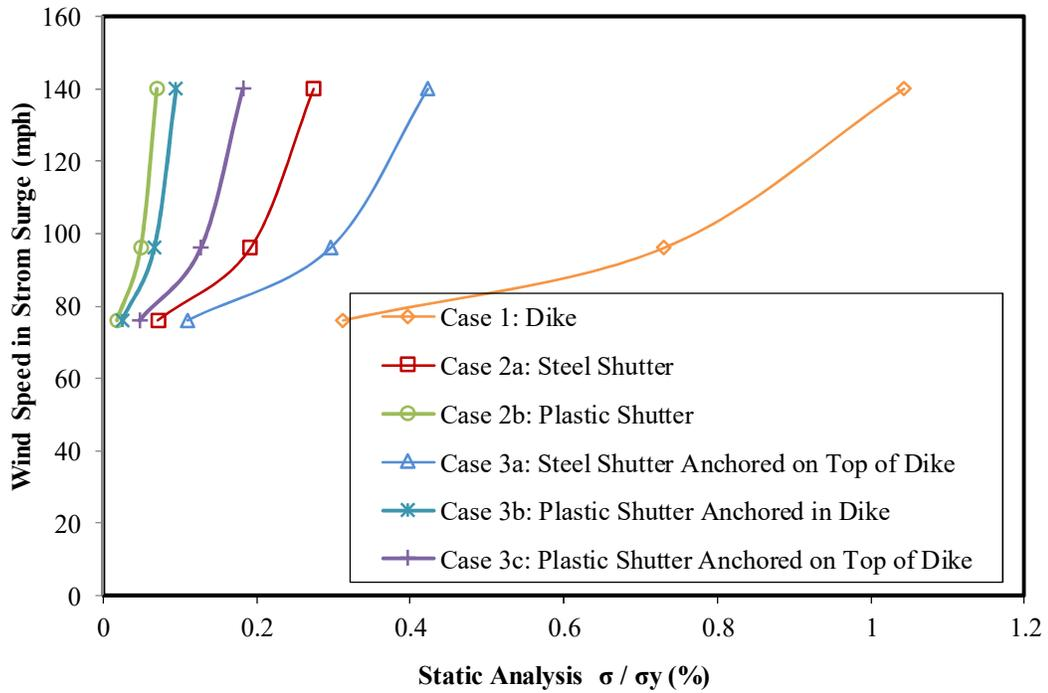
Figure 23: Wind speed versus normalized von misses stress for static analysis
