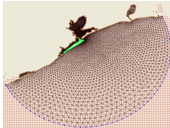
**Figure 5. Shoreline, ocean, bathymetry and mesh generation**
