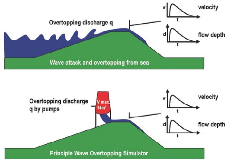
**Figure 2. Principle of the wave overtopping simulator**
