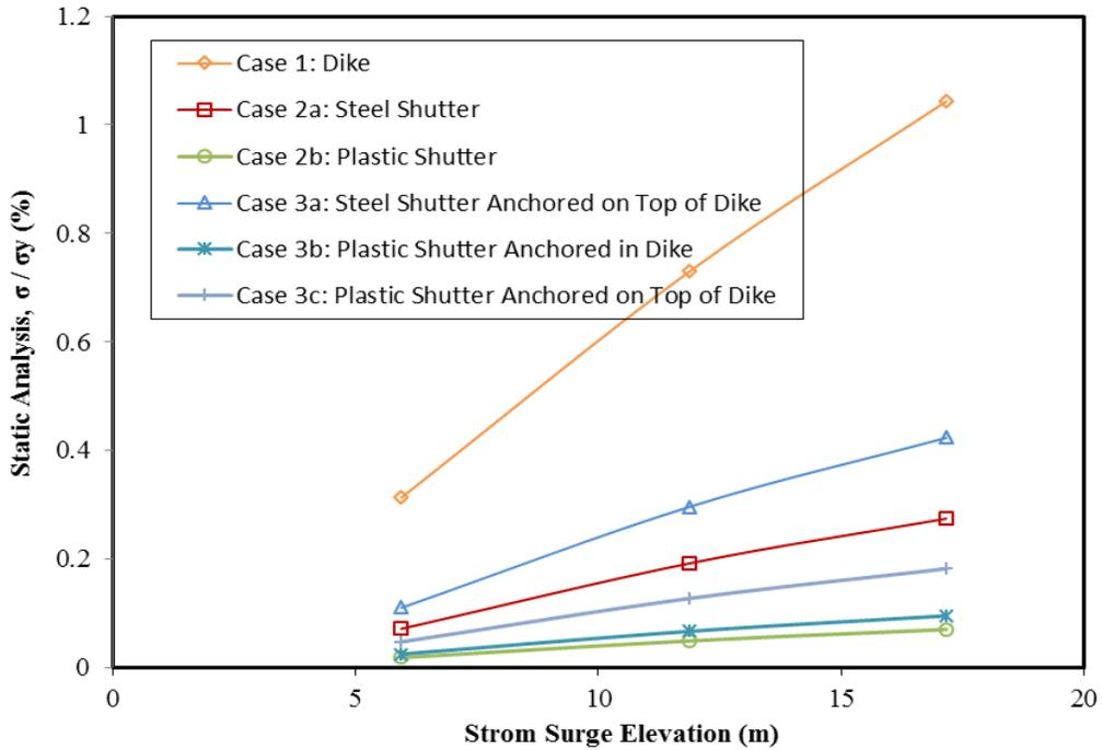
Figure 22: Normalized von misses from Static analysis versus storm surge elevation
