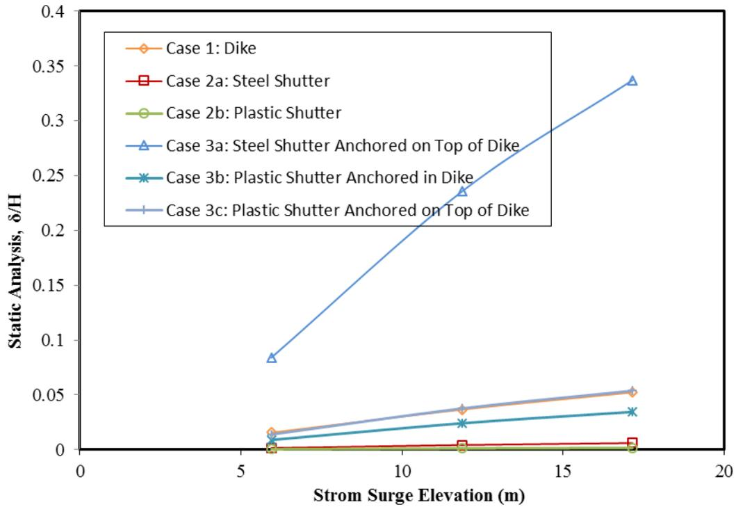
**Figure 21: Normalized displacement from Static analysis versus storm surge elevation**
