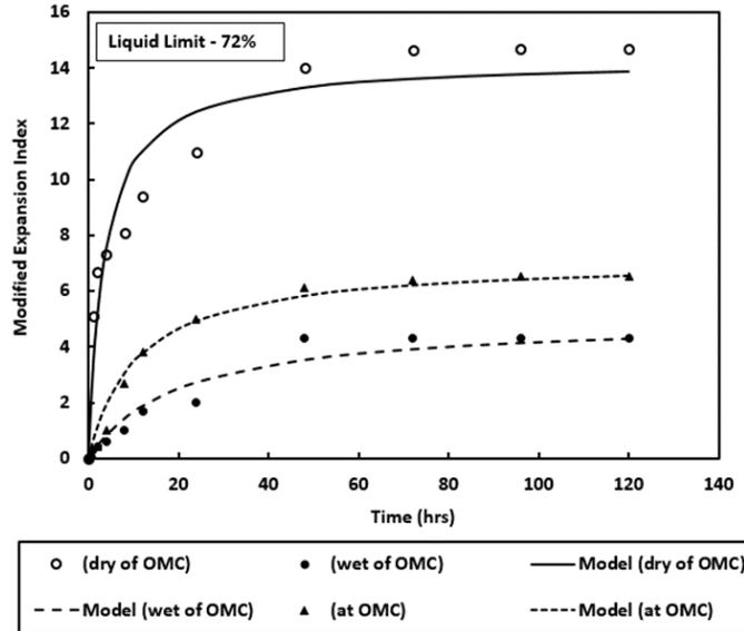
Figure 1. Variation of Modified Expansion Index with time for soils compacted at different moisture contents.
