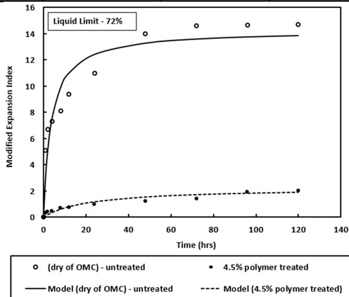
Figure 2. Modified Expansion Index after 4.5% pure polymer treatment.
