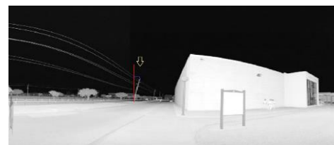
Figure-2: Manual registration of a pole at Lamar University, Beaumont, TX.
