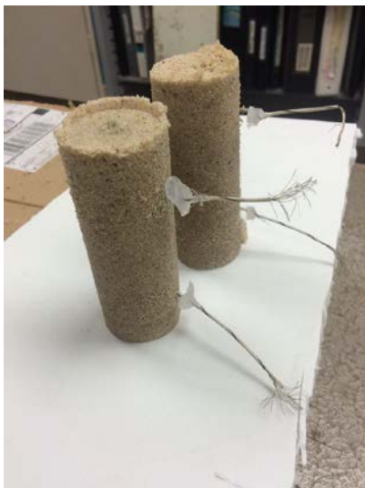
Figure 1. Grouted Sand Samples
