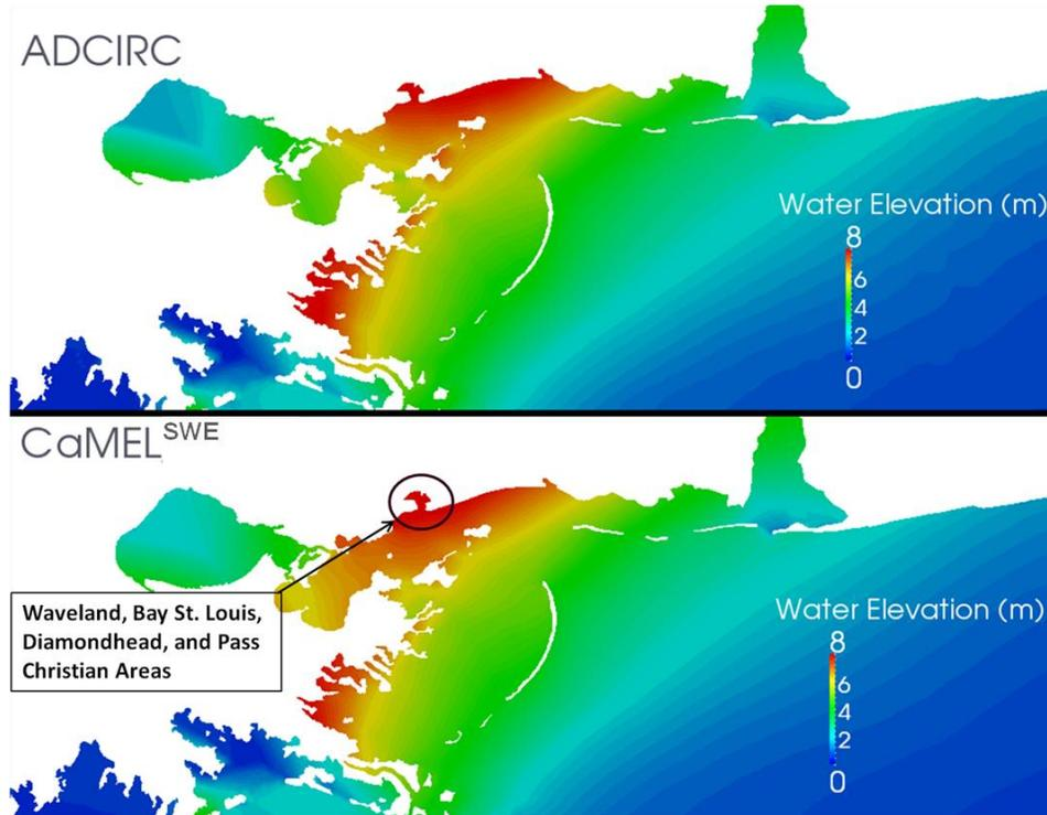
**Figure 3: Simulated maximum elevation of water (MEOW) comparison for ADCIRC and CaMEL<sup>SWE</sup>.**
