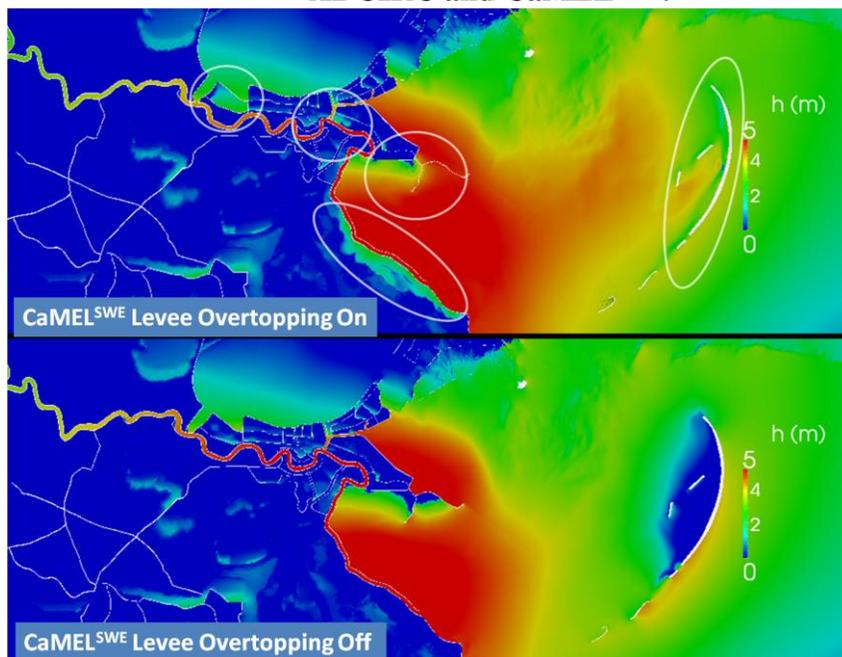
**Figure 4: Simulated results of New Orleans area levee and barrier overtopping using CaMEL<sup>SWE</sup> solver (Overtopped locations are pointed out by white ovals).**
